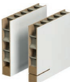
Preparation for shortening the door leaf • maximum 60 mm
